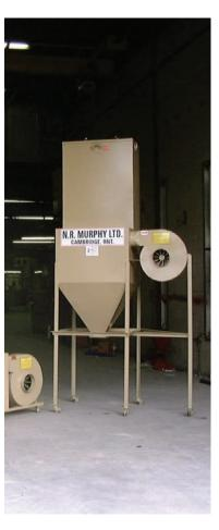
Check exhaust fan performance charts for required C.F.M. and resistance in N.R. Murphy Ltd.'s exhaust fan catalogue. NOTE: The C.F.M. mentioned in charts are a guide only. Please check with factory. Normal pressure drop allowance across units is 3" SP. N.R. Murphy Ltd. reserves the right to make changes to the information presented, product changes, and correct typographical errors without notice.
