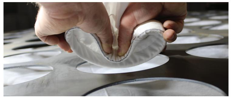
Insert folded tube into cell plate opening.
