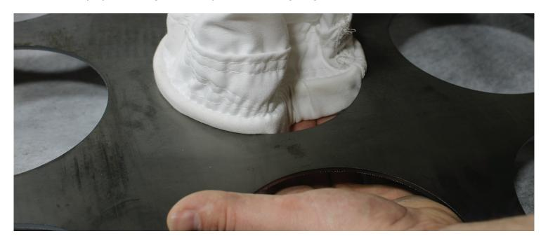
Please note, it is imperative the snap collars are securely fitted into the collar plate. The snap collars are designed with a indented ridge that will allow the filter to form a perfect seal. Filter collars not installed correctly will result in compromise of filtration, and the process may have to be restarted.
