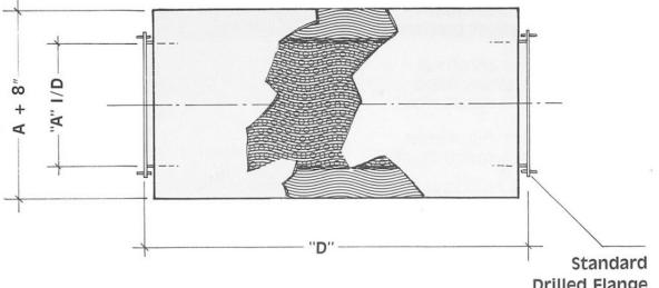
Drilled Flange Both Ends c/w Matching Flanges
